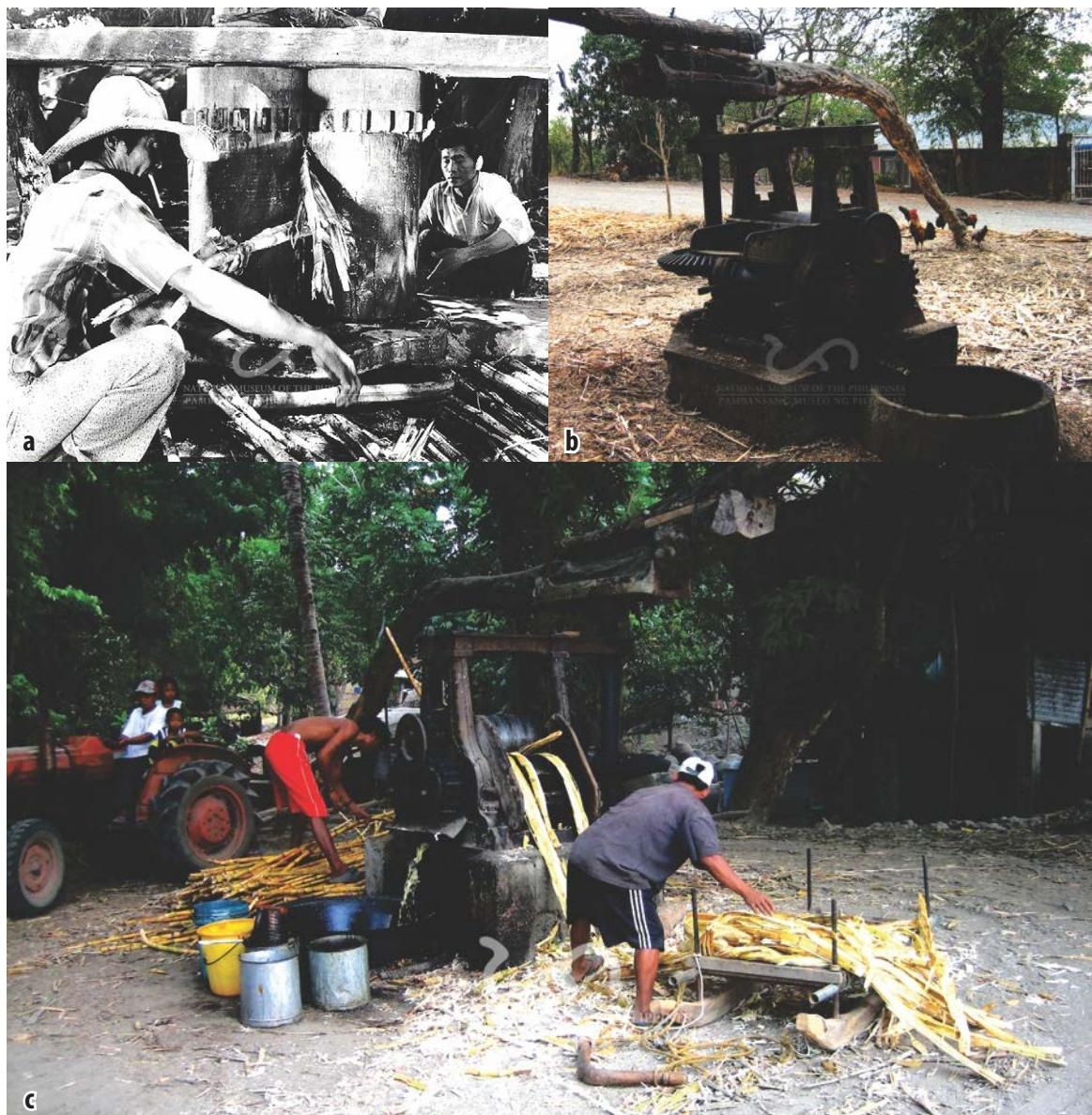
**Figure 1-3.** (a) Extracting *bennal* from the traditional *dadapilan*. 1980. Photographed by Dik Trofeo. Courtesy of the Filipinas Foundation, Inc. (b) One type of a metal *dadapilan*. (c) Extracting *bennal* from sugarcane in a tractor-powered *dadapilan*. Sarrat, Ilocos Norte | 2014. NMP Ethnology/MP Tauro.
